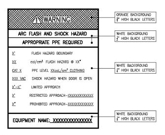
Label shall be orange and include the date of the study. Specify a second blue label to note arc-reduction levels, when using arc-flash reduction feature. Require manufacturer representative to provide a letter stating that they have visited the site and confirmed that the stickers have been applied in appropriate locations, per the approved Power System Study.
