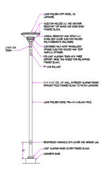
STANDARD WALKWAY LUMINAIRE AND POLE DETAIL
