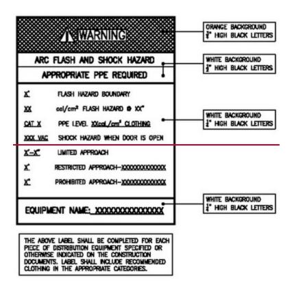
Label shall be orange and include the date of the study. Specify a second blue label to note arc-reduction levels, when using arc-flash reduction feature. Require manufacturer representative to provide a letter stating that they have visited the site and confirmed that the stickers have been applied in appropriate locations, per the approved Power System Study.
