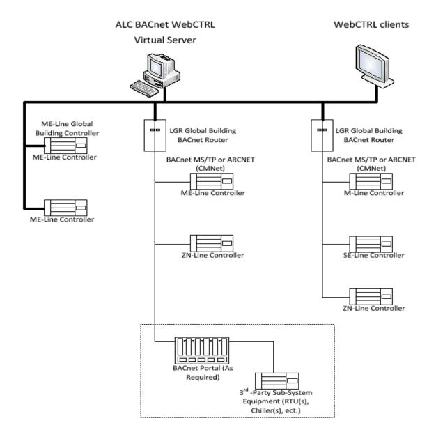
Figure 2: Building Automation System with Delta Controls product:
